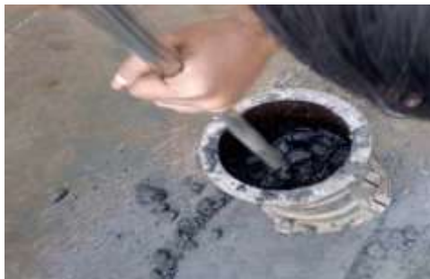
Placing of concrete in mould
